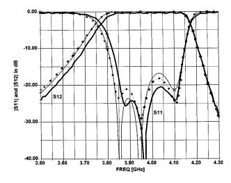
Fig. 7. Heavy solid lines show the measured response when for the filter in Fig. 1 the cover height is  $h_u = 3.810$  mm, while the dots show the measured response when the cover height is raised to 6.325 mm. The narrow solid lines shows the 3D planar CAD computed response for  $h_u = 6.325$  mm.
