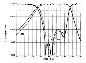
Fig. 5. Dots above show the measured response for the filter while the heavy solid lines show the response obtained utilizing 2D + 1 CAD with  $A_o = 25.6$  mm in Fig. 4 with  $f_{calc} = 3.95$  GHz (i.e., line parameters are calculated at the center of the passband). The narrow solid lines show the 2D + 1 CAD results if we replace  $A_o = 25.6$  with  $A'_o = 13.8$  mm in Fig. 4.
