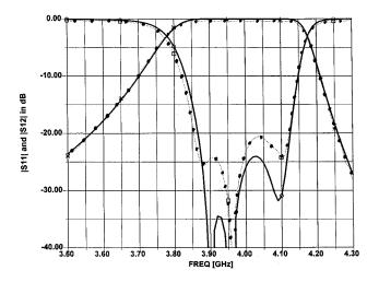
Fig. 6. Dots above show the measured response while the solid lines show the response computed using 2D + 1 CAD with  $A_o = 25.6$  mm as in the actual filter, but with the line parameter computed using  $f_{\rm calc} = 2.8$  GHz instead of 3.95 GHz.
