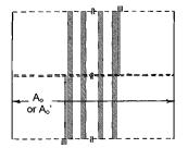
Fig. 4. Reinterpretation of the structure in Fig. 1 for use in an analysis program using 2D + 1 CAD. (Fringing capacitances, etc., must also be included.)
