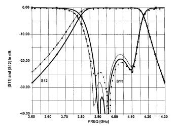
Fig. 2. Dots show the measured responses of the filter in Fig. 1 while the narrow solid lines show the 3D planar CAD results with the actual  $A_o = 25.6$ ,  $B_o = 51.2$  mm housing dimensions. The heavy solid lines show 3D planar CAD results if  $A_o = 12.8$ ,  $B_o = 25.6$  mm are assumed instead.
